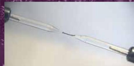
Fig. 3. Antenna of heather beetle suspended between electrodes for electroantennogram recording from receptors on antenna
