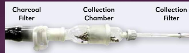
Fig. 2. Collection of volatile compounds from heather beetle. Air is drawn from left to right through a charcoal filter to purify it, through a glass chamber containing a heather beetle with heather and out through a collection filter which traps the volatile compounds for analysis
